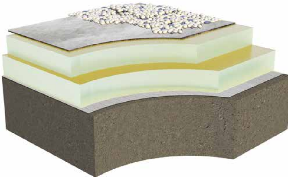
Warm roof (non-ventilated): Inverted roof
